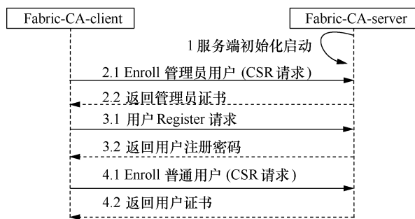
图 7 Fabric-CA 动态证书申请流程 Figure 7 The flowchart of dynamic certificate application for the Fabric-CA
